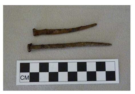
Image 11: (Top) machine cut nail (E115 N111) and (bottom) wrought nail (E115 N111).
